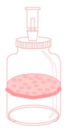
Microscale fermentation vessel (4 liters) • **Comparison of temperature control.** During the cold-soak, the commercial scale fermentation failed to reach the target temperature due to cooling inefficiency. In contrast, the microscale fermentation target temperature was easily achieved by controlling the temperature of the room.
