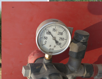
Bring up to RPM, spray out while noting pressure and time
