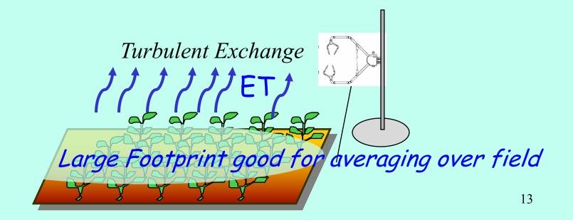
Vertical Turbulent Measurement of Gas Exchange using Sonic Anemometers and Gas Analyzers, 10 to 20 times a second-- "Eddy Flux" or "Eddy Covariance"
