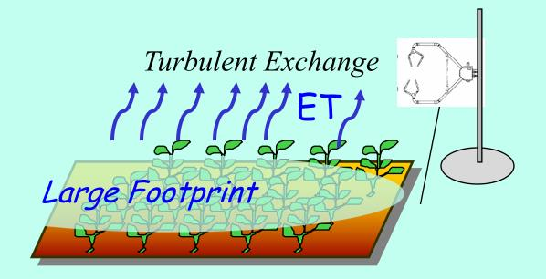
Vertical Turbulent Measurement of Gas Exchange using Sonic Anemometers and Gas Analyzers, 10 to 20 times a second: "Eddy Flux" or "Eddy Covariance"
