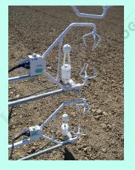
Vertical Turbulent Measurement of Gas Exchange using Sonic Anemometers and Gas Analyzers, 10 to 20 times a second: "Eddy Flux" or "Eddy Covariance"
