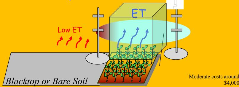
With Large Fields other Methods also: Aerodynamic Method, need wind speeds, relative humidity and temperature at two heights; look at decrease in humidity with height; challenges in measuring decreases because they can be small
